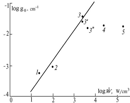
FIG. 2. Small-signal gain at  $\lambda = 585.3 \text{ nm}$  vs the excitation power. The numbers of close circles correspond to the line numbers in the table (see the text of this paper).
