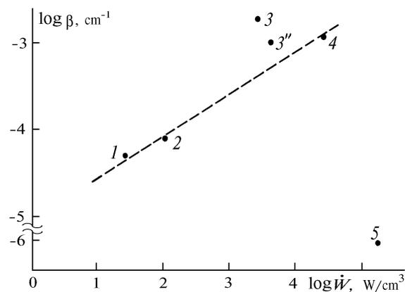
FIG. 3. Absorption coefficient at  $\lambda = 585.3 \text{ nm}$  vs excitation power. The numbers of close circles correspond to the line numbers in Table I (see the text of this paper).
