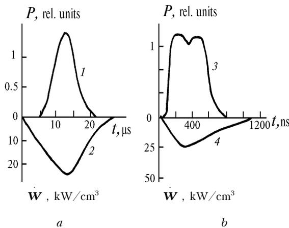
FIG. 1. Lasing pulse waveforms at  $\lambda = 585.3$  nm (1) and (3) and the temporal dependence of excitation power (2) and (4) for the mixtures He : Ne : Ar = 1.0 : 0.27 : 0.02 atm (a) and He : Ne : Ar = 2.1 : 0.34 : 0.06 atm (b).
