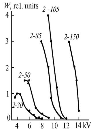
FIG. 3. Dependence of the lasing power at the 1.45- $\mu\text{m}$  neon line on voltage for the third-type device. The first number means the neon pressure and the second (after dash) – the helium pressure, capacitance is 0.4  $\mu\text{F}$ .
