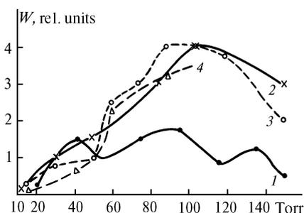
FIG. 4. Dependence of the maximum lasing power at the 1.45- $\mu\text{m}$  neon line on the helium pressure for the third type device. The neon pressure is 1 (1), 2 (2), 4 (3), and 8 Torr (4), and capacitance is 0.4  $\mu\text{F}$ .
