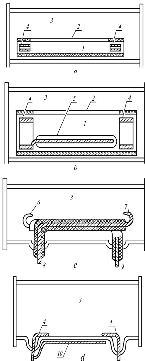
FIG. 1. Gas-discharge devices of the first (a), second (b), third (c), and fourth types (d). 1) ceramic tube, 2) slit, 3) chamber, 4) electrodes, 5) vitrified bar, 6 and 7) inside ends of electrodes forming the discharge gap, 8 and 9) outside ends of electrodes (leads), and 10) foil strip.
