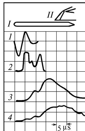
FIG. 2. Dynamics of the processes developing in the chamber of the first-type device. I is a photoscan schematic in tube and II is a photoscan schematic in the chamber. 1) Current, 2) lasing at the 2.026  $\mu\text{m}$  neutral xenon line in chamber, 3) spontaneous emission in chamber (588.9 nm neutral helium line), and 4) 840 nm neutral xenon line. Helium pressure is 150 Torr. Xenon pressure is 1 Torr, capacitance is 0.4  $\mu\text{F}$ , and voltage is 14 kV.
