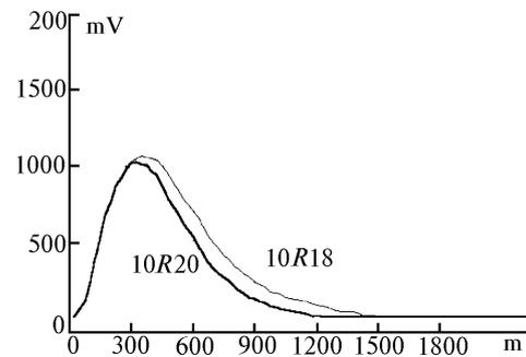
FIG. 2. Lidar returns for CO<sub>2</sub> laser lines 10R20(ON) and 10R18(OFF) obtained along horizontal path on October 20, 1989, 10:00 LT at air temperature of 18°C and relative humidity of 72%. The data are taken from Ref. 5.
