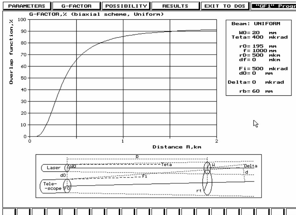
FIG. 3. Results of calculation by GF1 program: geometric parameters and geometric function of the lidar.
