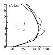
FIG. 5. Profiles of the tropospheric ozone concentration corrected for the aerosol contribution and derived from the data of multifrequency lidar at  $\lambda_{on} = 0.271 \,\mu\text{m}$  and  $\lambda_{off} = 0.289 \,\mu\text{m}$ : 1) profile obtained by the differentiation algorithm, 2) exact profile, and 3) profile obtained by the differential scheme.
