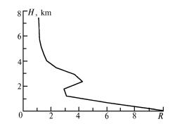
FIG. 4. Profile of the scattering ratio obtained when sounding the troposphere at a wavelength of  $0.532 \ \mu m$ .
