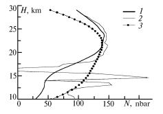
FIG. 1. Ozone concentration profiles obtained without their correction for aerosol contribution at  $\lambda_{on} = 0.308 \ \mu\text{m}$  and  $\lambda_{off} = 0.353 \ \mu\text{m}$ : 1) exact profile, 2) profile obtained by differential scheme, and 3) profile obtained by the algorithm of differentiation of empirical dependence.
