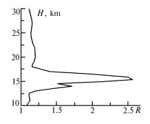
FIG. 2. Profile of the scattering ratio at a wavelength of  $0.532 \ \mu m$  obtained when sounding the stratosphere.
