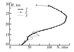
FIG. 3. Profiles of the stratospheric ozone concentration corrected for aerosol contribution and derived from the data of multifrequency lidar at  $\lambda_{on} = 0.308 \ \mu m$  and  $\lambda_{off} = 0.353 \ \mu m$ : 1) exact profile, 2) profile obtained by the differentiation algorithm and 3) profile obtained by the differential scheme.
