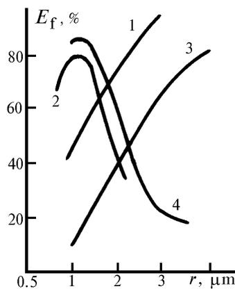
FIG 1. Efficiency of catching particles of different size in a human nasal cavity (1), in alveoles (2) and on third and fourth cascades of an impactor (curves 3 and 4, respectively).
