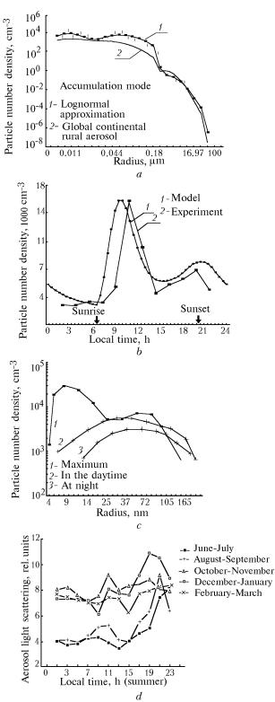
FIG. 3. Size spectrum of aerosols in Siberia (a); dynamics of the diurnal variations of the number density of the submicron fraction of atmospheric aerosol particles in Siberia, experimental and theoretical data (b); dynamics of variations of the size spectrum of the submicron aerosol fraction (c); seasonal variations of the diurnal behavior of light scattering by the submicron fraction (d).
