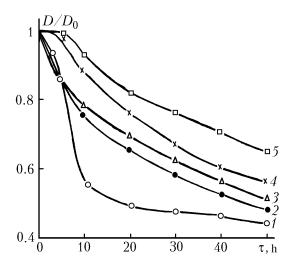
FIG. 1. Kinetic decolorization curves of rhodamine 6G in the MMA-MAA copolymer with modifying dopants: without dopants (1), with HMDU (2), DPU (3), DPTU (4), and PBTU (5). Dopant concentration is 0.004 mole %.
