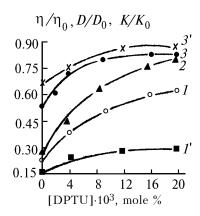
FIG. 2. Functions of relative viscosity change  $\eta/\eta_0$  of colored MMA-MAA copolymer solutions (1, 1'), phototransmission coefficient  $K/K_0$  of a colorless copolymer (2), and optical density of dyes  $D/D_0$  in a copolymer (3, 3') after 20 hours of radiation on the DPTU concentration in copolymer: rhodamine 6G (1, 3); coumarin 7 (1', 3').
