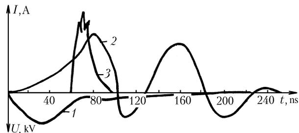
FIG. 3. Oscillograms of the pulses of voltage (1), current (2), and power of lasing (3) (net power at both lasing lines of the copper vapor laser).
