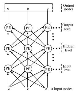
FIG. 2. Multilevel neural network structure
