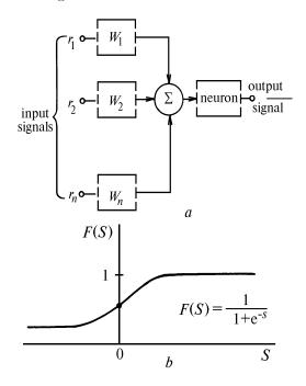
FIG. 1. Processor element structure (a) and sigmashaped neuron function (b).
