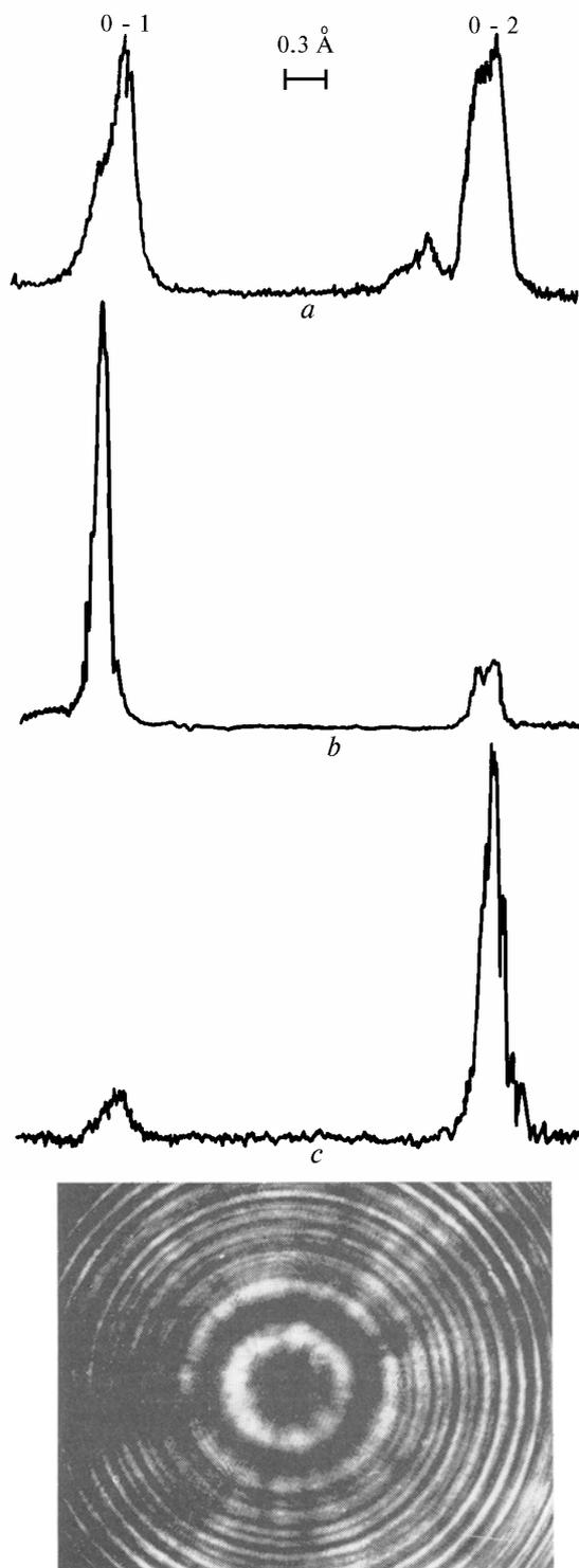
FIG. 2. Densitograms of the output spectra in the free-running mode (a) and injection seeded mode with the injection into 0-1 transition (b) and 0-2 transition (c). Interferogram of the output spectrum of the laser emission in the injection seeded mode (d)
