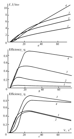
FIG. 4. a) Total (at  $\lambda_1=351$  and  $\lambda_2=353$  nm) emitted energy vs ionization frequency in optimal mode of lasing, the Ne–Xe–NF3 mixture, p=1 atm, for the pump duration at half–maximum  $\tau_{1/2}=1$  (curve 1), 0.4 (curve 2), 0.2 (curve 3), and 0.1 ms (curve 4);
