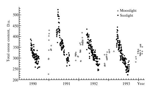
FIG. 1. Measurement results on the total ozone content at Heiss Island in 1990–1994.
