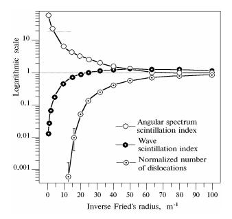
FIG. 2. Estimates of scintillation indices of wave and its angular spectrum and normalized number of wave phase dislocations. Standard deviations are indicated as confidence intervals. These deviations are not indicated if their values are less than point size.
