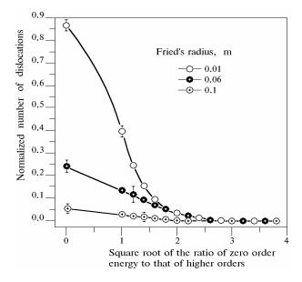
FIG. 3. Phase dislocation suppression due to amplification of the zero order of a wave. Standard deviations are indicated as confidence intervals. These deviations are not indicated if their values are less than point size. Zero abscissas correspond to the case in which the zero order was not changed.
