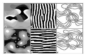
FIG. 1. Wave phase dislocations and structures created by them. Crosses denote zeros of the intensity and corresponding points of phase dislocations: wave intensity (a); wave phase (b); interference pattern for unit amplitude and carrier wave perpendicular to horizontal coordinate axis (c); interference pattern for unit amplitude and carrier wave perpendicular to vertical coordinate axis (d); contour lines of phase sine (e); and, contour lines of phase cosine (f).
