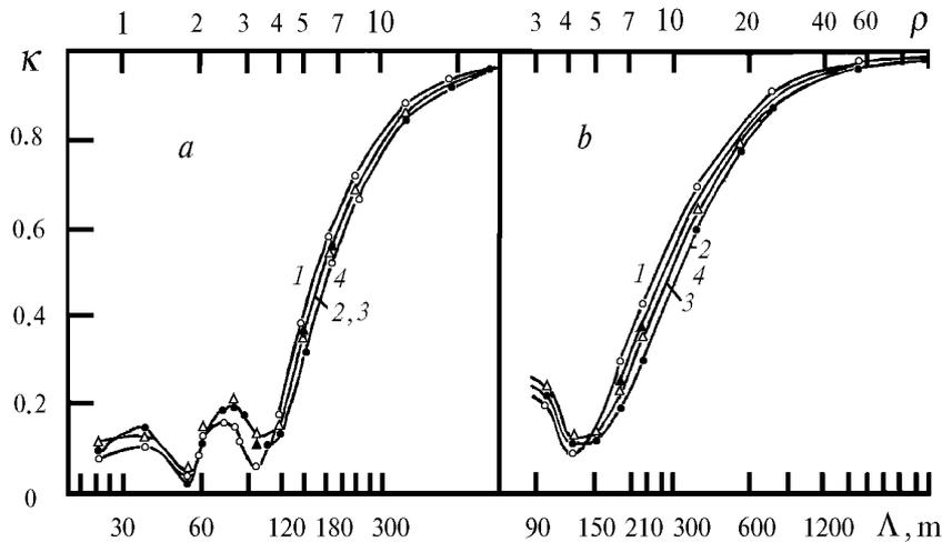
FIG. 1. A sample calculation of AFC of the laser sensing channel for a remote cloud layer with the optical density increasing along the probing direction. The optical thickness of the cloud layer  $\tau = 2$  (a) and 4 (b). The curve numbers correspond to the detector angles of vision in the  $3'$ – $3^\circ$  range.
