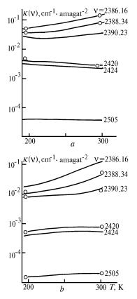
FIG. 2. Temperature dependence of the  $CO_2-CO_2$  (a) and  $CO_2-N_2$  (b) absorption coefficients in the 4.3 µm band at several frequencies given to the right of the curves.
