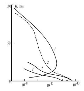
FIG. 4. Altitude dependence of the weighting function at dT/dz for several frequencies: v = 2360.8 (1), 2379.27 (2), 2392.35 (3), and 2424 cm<sup>-1</sup> (4).
