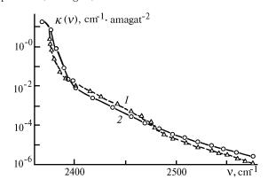
FIG. 1. The CO<sub>2</sub> absorption coefficient in the 4.3 µm band wing at T = 193 K (curve 1) and at T = 296 K (curve 2) calculated on the basis of the line wing theory. Experimental data are taken from Ref. 6: o - 296 K and  $\Delta - 193$  K.
