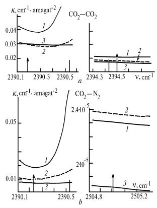
FIG. 3. Change in the character of the temperature dependence of the CO<sub>2</sub>-CO<sub>2</sub> (a) and CO<sub>2</sub>-N<sub>2</sub> (b) absorption coefficients in the vicinity of several sensing channels (marked by arrows). The curves correspond to temperatures of 300 (1), 250 (2), and 190 K (3).
