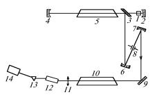
FIG. 1. Diagram of the setup for conversion of CVL emission in nonlinear crystal.
