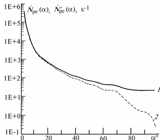
FIG. 3. The angular distribution of brightness at a distance of 5 m from a Lambertian source of light (the Lake Baykal 1-km depth): counting rate of photon pulses  $\dot{N}_{pe}(\alpha)$  measured with a PMT–130 (1), calculations of  $\dot{N}'_{pe}(\alpha)$  (2).
