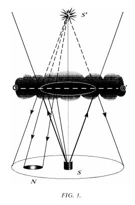
In this experiment we used a floodlight setup in which arc xenon superhigh-pressure lamps DKSSh-4000 were used as an emitter. The spherical mirror was 500 mm in
