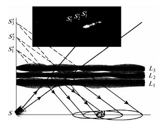
FIG. 3. Fragment of video frame (removed at a 100 m distance from the floodlight) and scheme of complicated reflection formation during slant sounding: S - floodlight, N - observer,  $S'_1$ ,  $S'_2$ , and  $S'_3$  are virtual images of the floodlight on the reflecting layers  $L_1$ ,  $L_2$ , and  $L_3$ .
