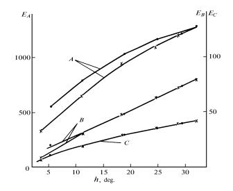
FIG. 1. Energy density of the UV irradiance as a function of the solar elevation angle for spectral ranges A, B, and C (March 16, 1993). Points are for sunrise, and crosses are for sunset.
