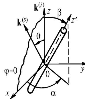
FIG. 1. Geometry of scattering by arbitrarily oriented circular cylinder.
