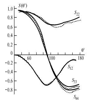
FIG. 2. Angular dependences of the normalized components of the model scattering phase matrices  $S(\theta)$ .  $S_1$  is shown by solid lines,  $S_2$  is shown by points.
