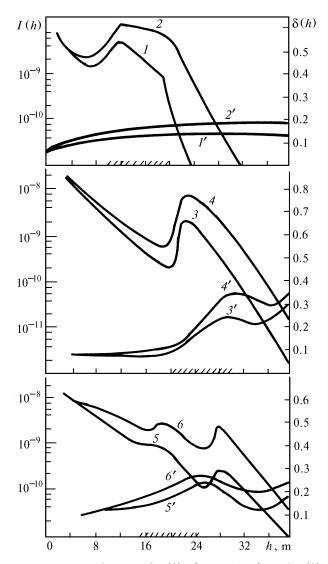
FIG. 4. Dependences of I(h) (curves 1–6) and  $\delta(h)$  (curves 1'–6') in the presence of the submerged inversion layers with different stratification.  $\varphi_d = 5$  (1, 3, and 5) and 10 mrad (2, 4, and 6).
