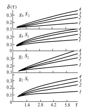
FIG. 3. Dependence of the depolarization ratio on the sounding depth for media that differ in their scattering properties.  $\varphi_d = 5$  (1), 10 (2), 20 (3), and 35 mrad (4).
