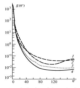
FIG. 1. Angular dependences of the scattering phase functions  $g_1(\theta), \ldots, g_4(\theta)$  indicated by the numbers adjacent to each currve.
