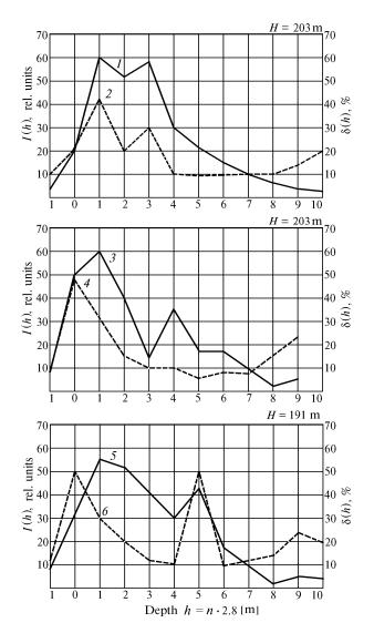
FIG. 5. Experimentally measured dependences of I(h) and  $\delta(h)$  for different regions of the Barents Sea. I(h) is illustrated by solid curve and  $\delta(h)$  — by dashed curve.
