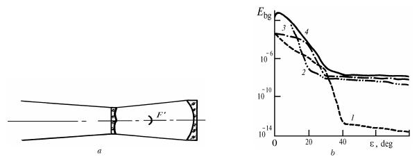
FIG. 2. The Schmidt mirror-lens objective and a) optical scheme of the objective; b) ambient background illumination in the focal plane of the optical system vs the angle of incidence of input radiation. Contributions of diffraction (1), scattering (2), and re-reflection of radiation (3) in the optical system to the ambient background illumination and the total ambient background illumination vs the angle of incidence of input radiation (4).
