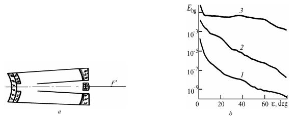
FIG. 1. The mirror-lens MTO-1000 A objective. a) optical scheme of the objective and b)ambient background illumination in the focal plane of the optical system vs the angle of incidence of input radiation. Contributions from diffraction (1), scattering (2), and re-reflection (3) of radiation in the optical system to the ambient background illumination.
