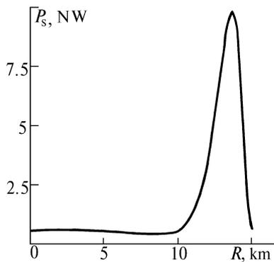
FIG. 4. A reference model of a signal;  $P_s$  – the optimal power of the signal, NW and  $R$  – the distance between a 15–km atmospheric layer and the Earth’s surface, km.
