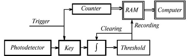
FIG. 3. A functional block-diagram of the processing of a signal.
