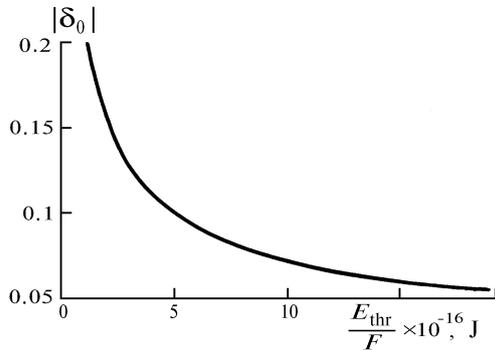
FIG. 1. The absolute value of the relative error  $\delta_0$  of recovering the sum of optical power of a signal and background  $P(t)$  as a function of the relation between the threshold energy  $E_{thr}$  and the PMT's noise coefficient  $F$ .
