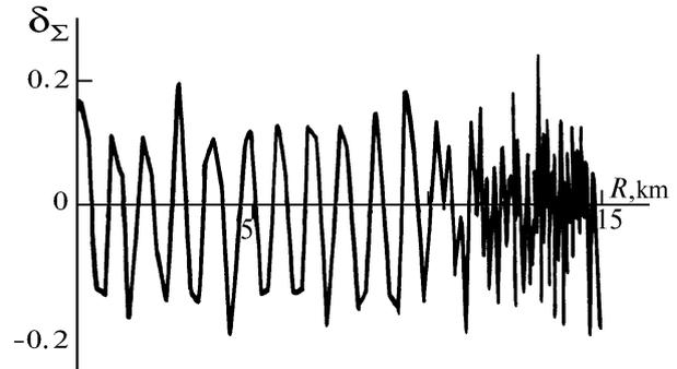
FIG. 5. A relative error  $\delta_\Sigma$  of recovering the initial signal;  $q_{\text{min}} = 1$ ,  $R$  is the distance between a 15–km atmospheric layer and the Earth’s surface, km and  $E_{\text{thr}} = 15.6 \cdot 10^{-16}$  J.
