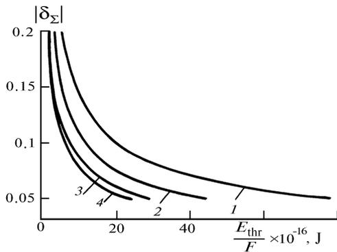
FIG. 2. The absolute value of the relative error  $\delta_\Sigma$  of recovering the optical power of a signal ( $P_s$ ) as a function of the relation between the threshold energy  $E_{thr}$  and the PMT's noise coefficient  $F$ : 1)  $q_1 = 1$ , 2)  $q_1 = 3$ , 3)  $q_1 = 5$ , and 4)  $q_1 = 10$ .
