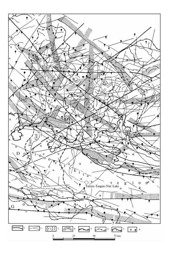
FIG. 3. A structure-hydrogeological scheme of the central part of the Dolinoozerski artesian basin of Mongolia (based on the results obtained from a synthesized satellite picture, spacecraft "Salyut-6", July 24, 1982). 1–4) breaking destructions: 1) regional depth breaks, 2) other breaks, 3) ring structures, and 4) zones of fracturing. 5–7) boundaries of: 5) the Dolinoozerskii artesian basin, 6) water-catch river basins, 7) regional areas of supply, and 8) water manifestation (holes, springs).
