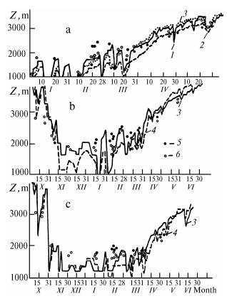
FIG. 1. Altitude position of a snow line for the basins of the Gavasai river, in 1978 (a) and in 1983 (b); the Kassansai river, in 1983 (c). The calculational results obtained using a model for six-hour (1) and day (2-4) intervals and the results of the analysis of satellite data: 1) and 3) using formula (1),  $K_1 = 5 \text{ mm/(deg-day)}$ ; 2) using formula (2),
