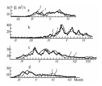
FIG. 2. Actual (1) and calculated using  $K_1 = 5 \text{ mm/(deg-day)}$ , (2), hydrographs of the Gavasai river outflow – mountain settlement Gava: a) 1975, b) 1980, and of the Kassansai river – mountain settlement Kyzyltokoi: c) 1980, d) 1982.
