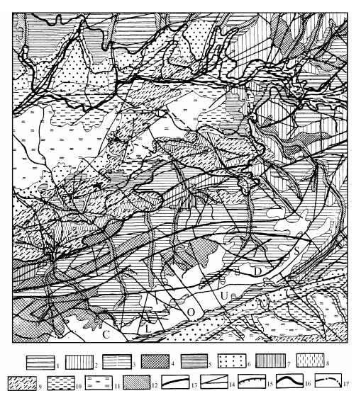
FIG. 4. Hydrogeodynamic scheme of conditions of forming underground waters in the Eastern part of the Fergana artesian basin (results of analysis of satellite pictures taken from an artificial satellite of the Earth "ERTS-1", June 4, 1973).
