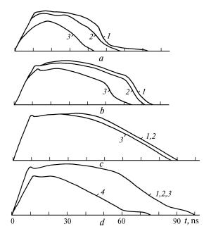
FIG. 1. Oscillograms of output pulses from the LIDA-T laser with a 3.5 cm electrode separation and surface discharge irradiation using  $C_1$  and  $C_2$ : a) He:KrHCl = 2.75 atm: 125 Torr: 3 Torr, b) Ne:KrHCl = 5 atm: 125 Torr: 3 Torr, c) He:Xe:HCl = 3 atm: 30 Torr: 3 Torr, d) Ne:Xe:HCl = 5 atm: 30 Torr: 3 Torr,  $U_0 = 40$  (1), 35 (2), 30 (3), and 25 (4) kV.
