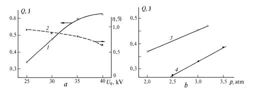
FIG. 3. The radiation energy (1) and efficiency (2) as a function of charge voltage (a) and the radiation energy as a function of mixture pressure (b) at charge voltage 30 (3) and 40 kV (4). 1, 2, 3) discharge circuit inductance  $L_0 = 10$  nH, 4)  $L_0 = 220$  nH.  $C_0 = 120$  nF,  $C_1 = 3.3$  nF.
