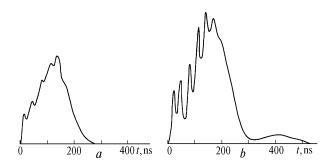
FIG. 4. Oscillograms of lasing pulses produced at  $U_0 = 40$  kV,  $C_0 = 120$  nF,  $C_1 = 3.3$  nF with a mixture of Ne : Xe : HCl = 2.5 atm : 12 Torr : 3 Torr.  $L_0 = 107$  (a) and 190 nH (b).
