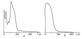
FIG. 5. Oscillograms of lasing pulses produced at  $U_0 = 40$  kV,  $C_0 = 120$  nF,  $L_0 = 220$  nH with a mixture c Ne : Xe : HCl = 3.5 atm: 15 Torr : 3 Torr.  $C_1 = 7.3$  (a) an 13.3 nF (b).
