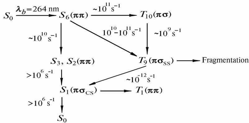
FIG. 3. Scheme of photodissociation mechanism of disulfide molecules.
