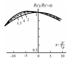
FIG. 2. The echo pulse received from a randomly rough surface with a combined scattering phase function sounded through the optically dense atmosphere.
