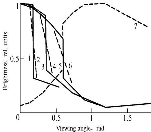
FIG. 3. Normalized brightness distribution over the input pupil of the OES.  $z_{st} = 0.01$  m: 1)  $h = 100$  m,  $\sigma^2 = 0$ ; 2)  $h = 100$  m,  $\sigma^2 = 0.2$ ; 3)  $h = 50$  m,  $\sigma^2 = 0$ ; 4)  $h = 50$  m,  $\sigma^2 = 0.2$ ; 5)  $h = 30$  m,  $\sigma^2 = 0$ ; 6)  $h = 30$  m,  $\sigma^2 = 0.2$ , and  $z_{st} = 0.51$  m, and 7)  $h = 30$  m,  $\sigma^2 = 0$ .
