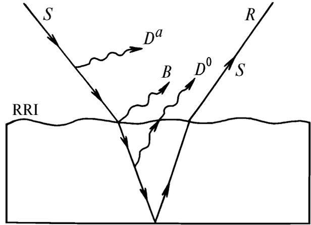
FIG. 2. Structure of the optical signal in the OES of observation. Here  $D^a$  is the haze of the atmosphere,  $D^0$  is the haze of the ocean,  $B$  is the glint reflection from the RRI, and  $S$  is the valid signal.
