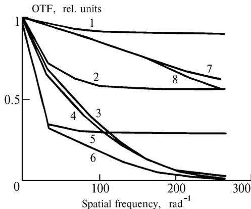
FIG. 4. Optical transfer function of the OES of observation.  $h = 30$  m. Narrow beam: 1)  $z = 1$  m,  $\sigma^2 = 0$ ,  $\rho_0 = 0$ ; 2)  $z = 3$  m,  $\sigma^2 = 0$ ,  $\rho_0 = 0$ ; 3)  $z = 3$  m,  $\sigma^2 = 0.2$ ,  $\rho_0 = 0$ ; 4)  $z = 3$  m,  $\sigma^2 = 0.2$ ,  $\rho_0 = 0.5$ ; 7)  $z = 1$  m,  $\sigma^2 = 0.2$ ,  $\rho_0 = 0$ ; 8)  $z = 1$  m,  $\sigma^2 = 0.2$ ,  $\rho_0 = 0.5$ . Plane wave: 5)  $h = 3$  m,  $\sigma^2 = 0$  and 6)  $z = 3$  m,  $\sigma^2 = 0.2$ .
