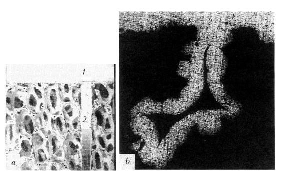
FIG. 4. Photomicrograph of the experimentally realized structure of the composite copper substrate of the active mirror: a) compact layer (substrate of the mirror) (1) and model of the actuator case (2) and b) joint of the compact substrate of the specular surface and the elastic permeable sublayer fabricated from the HPM.
