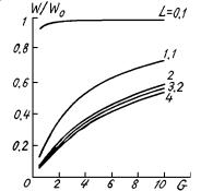
FIG. 3. The family of the dependencies of the displacement  $W/W_0(G)$  of the actuator transferred through the layered substrate of the active mirror on the relative stiffness of the actuator G for different values of L.
