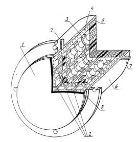
FIG. 1. The diagram of the active spherical mirror.
