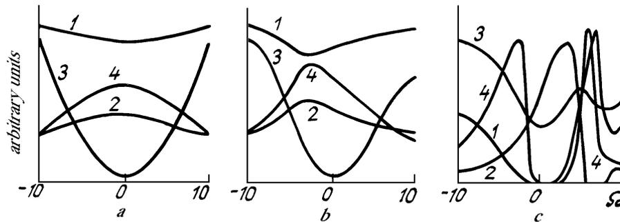
FIG. 2. The time dependences of the lasing power (1), the difference between the populations of the working levels of the active medium (2), and the populations of the lower (3) and upper (4) levels of the absorbing medium: a)  $\varepsilon = 0$ ; b)  $\varepsilon = 5 \cdot 10^{-3}$ ; c)  $\varepsilon = 2 \cdot 10^{-2}$ . The rest of the parameters are the same as in Fig. 1.
