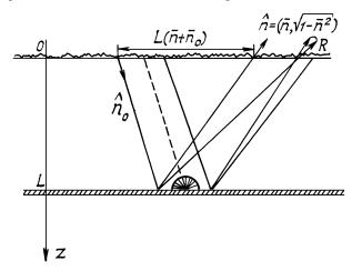
FIG. 2. Reflection of the paraxial beam from the layer of the diffuse scatterers in the homogeneous medium: Unperturbed porblem.
