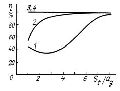
FIG. 1. The normalized criterion of correction quality  $\eta$  as a function of the radius  $S_t$  of the receiving aperture for different number of the controllable modes. 1) without correction, 2) second-order modes, and 3, 4) third- and fourth-order modes, respectively. Path length  $z_0 = 0.5$  and the nonlinearity parameter R = -20.
