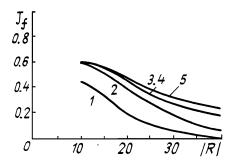
FIG. 3. The criterion of focusing  $J_f$  within the circle of radius  $S_t = 2a_d$  as a function of. the nonlinearity parameter R. 1) without correction, 2) second—order mode, 3, 4) third—and fourth—order modes, respectively, and 5) ideal corrector. Path length  $z_0 = 0.5$ .
