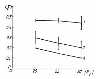
FIG. 4. The resultant values of the criterion of focusing J averaged over 30 iterative steps vs the nonlinearity of the medium in the case of stationary refraction at  $z_0 = 0.5 z_d$ . 1) two-mirror system, 2) phase conjugation and 3) without control.
