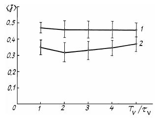
FIG. 5. Adaptive control in the presence of pulsations of the wind velocity. The quality of correction of thermal blooming vs the period of wind velocity pulsations  $T_v$  $z_0 = 0.5 z_d$  and  $\langle R \rangle = -20$ . The interval of time averaging is about 40  $\tau_v$ . 1) adaptive two-mirror system and 2) algorithm of cross-aperture sensing.
