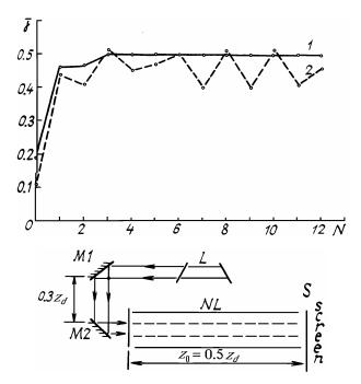
FIG. 1. Compensation for thermal blooming based on the PC algorithm in the case of stationary wind refraction. J is the focusing criterion, N is the number of iterative steps, and  $z_0 = 0.5 z_{d}$ . 1)  $|R_v| = 20$  and 2)  $|R_v| = 30$ .
