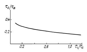
FIG. 2. The dependence of the ratio  $\tau_d/\tau_a$ , at which the maximum speed is attained in the inertial adaptive system, on the inertial time delay  $\tau_i/\tau_d$ .
