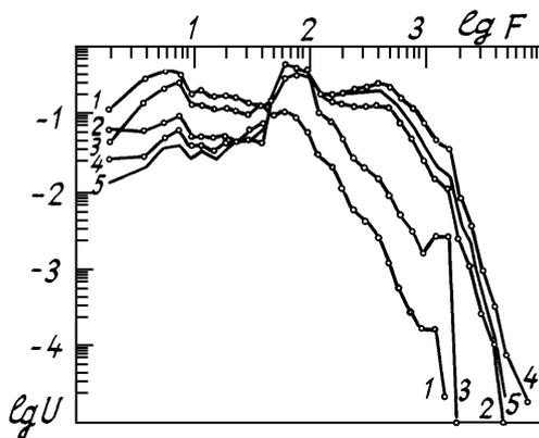
FIG. 3. Intensity fluctuation spectrum  $U(f) = \frac{w(f)}{\int w(f)df}$  where  $w(f)$  is the spectral density at frequency  $f$  with different slit displacements from the center of diffraction pattern ( $y$  is in  $\mu\text{m}$ ) 1) 0, 2) 60, 3) 25, 4) 85, and 5) 110.
