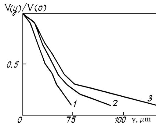
FIG. 1. Distribution of the mean intensity over the focal plane of the receiving lens at different values of optical depth  $\tau$ : 1) 0.6, 2) 3.1, and 3) 3.9.
