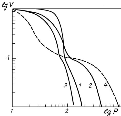
FIG. 2. Dependence of the function  $V(p)$  on the parameter  $P = 2\kappa Ry/F$  at different  $\tau$ , where  $\kappa = 2\pi/\lambda$ ,  $R$  is the lens radius,  $F$  is the focal length, and  $y$  is the slit displacement. 1) 0, 2) 4.3, 3) 0.9, and 4) 2.4 calculation.<sup>2</sup>
