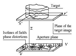
FIG. 1. Target, aperture, and field of phase distortions.
