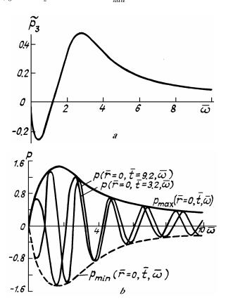
FIG. 4. Frequency dependence of the amplitude of the periodic component of the acoustic response on the beam axis (a) and the dependence of the maximum (solid lines) and minimum (dashed lines) sound pressures on the beam axis on the modulation frequency (b).
