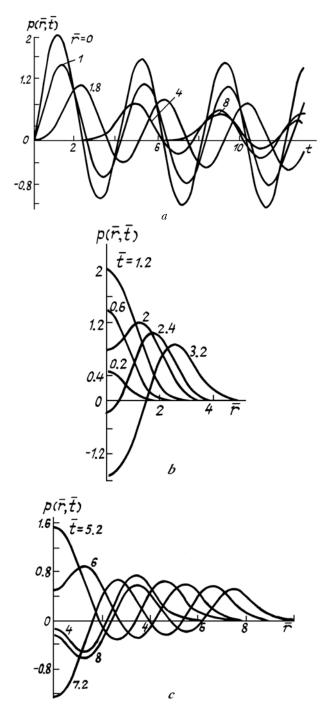
FIG. 3. Temporal behavior of the sound pressure at various distances  $\overline{r}$  from the beam axis for harmonic modulation of the beam intensity with the frequency  $\overline{\omega} = 1.6$  (a). Distances from the beam axis are indicated on the curves. Changes in the sound pressure with distance at different times  $\overline{t}$  indicated on the curves (b and c).
