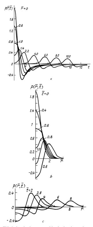
FIG. 2. Sound pulses generated by the short laser pulse at various distances from the beam axis  $\overline{r}$  indicated on the curves (a) and sound fields generated by the same pulse at different times  $\overline{t}$  indicated on the curves (b and c).
