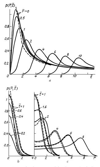
FIG. 1. Sound pulses generated by the stepwise leading front of laser signal at various distances from the beam axis  $\overline{r}$  indicated on the curves (a) and sound fields generated by
