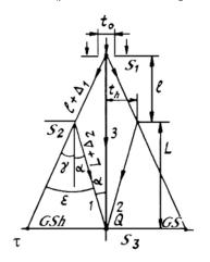
FIG. 1. The diagram of interference of the rays diffracted by the edges of a slit of the variable width with the axial rays.
