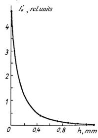
FIG. 2. The intensity of the edge rays on the beam axis as a function of the distance between the observation point and shadow boundary formed by the screens of a slit of the variable width.
