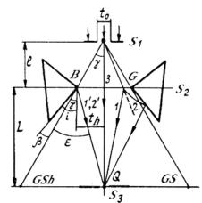
FIG. 3. The diagram of amplification of the intensity of the edge rays on the light beam axis.
