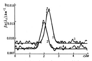
FIG. 2. Numerical simulation of processing of bifrequency sounding data with the help of the proposed algorithm at  $\tau \approx 1$ ; 1), 2) model profiles of  $\beta(\lambda_i, z)$ , and 3), 4) the reconstructed profiles.
