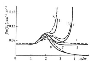
FIG. 1. Examples of the instability of the solutions caused by the error  $\Delta\beta(\lambda_i, 0)$  at the reference point  $z_p = 0$ . Curves 1 and 2 represent model profiles of  $\beta(\lambda_i, z)$  and 3 and 4 represent the reconstructed profiles.  $\Delta\beta(\lambda_i, 0) = 0.5$  (3 and 4), 2 (5 and 6), and -2% (7 and 8).
