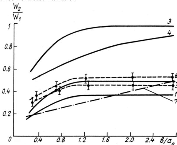
FIG. 2. Dependence of the correction-accuracy parameter on the normalized radius of the receiving aperture of the mirror for fixed  $\varphi_0$  and  $\rho_0$  and different  $d$ . 1–4, 7) computations and 5, 6) experiment.
