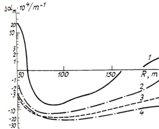
FIG. 2. The turbulence-wind shift in the difference of the sound absorption coefficients with a wind velocity of  $5 \text{ m} \cdot \text{s}^{-1}$ .
