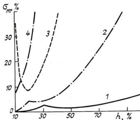
FIG. 4. The absolute error in measuring the relative humidity at a height of 100 m in the presence of wind with a velocity of  $5 \text{ m} \cdot \text{s}^{-1}$ .
