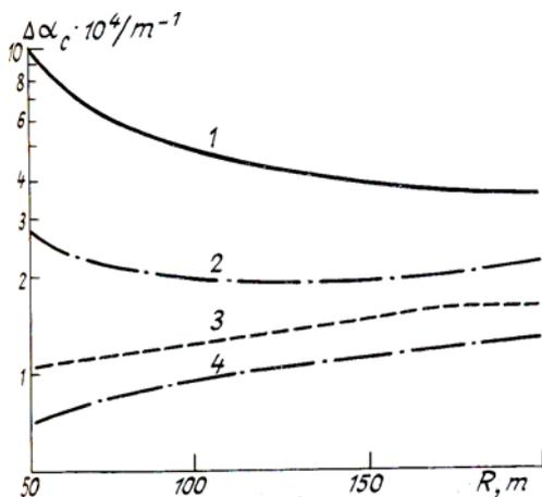
FIG. 1. The turbulent shift in the difference of the sound absorption coefficients under almost calm conditions.
