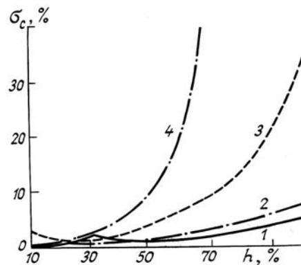
FIG. 3. The absolute error in the measurement of the relative humidity under almost calm conditions (the height is equal to 100 m).
