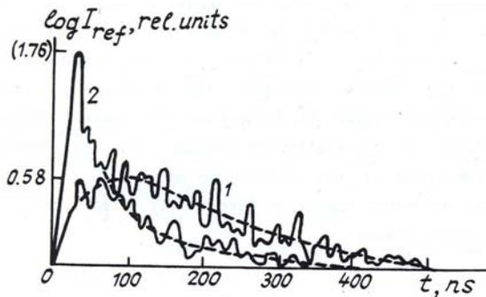
FIG. 2. Densitometer traces of the shape and intensity of the reflected signal with different extinction factors of the scattering medium:  $\epsilon_{\min} = 56.6 \text{ m}^{-1}$  (1), and  $\epsilon_{\max} = 3600 \text{ m}^{-1}$  (2). The dashed lines show the average value of the densitometer tracings.
