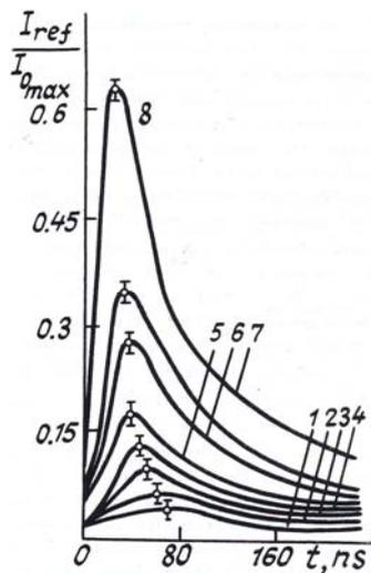
FIG. 3. Densitometer traces of the shape and intensity of the reflected signal scaled to the maximum intensity of the sounding pulse (on a linear scale) for different  $\epsilon$ :  $56.6 \text{ m}^{-1}$  (1),  $73 \text{ m}^{-1}$  (2),  $115 \text{ m}^{-1}$  (3),  $186 \text{ m}^{-1}$  (4),  $257 \text{ m}^{-1}$  (5),  $506 \text{ m}^{-1}$  (6),  $1200 \text{ m}^{-1}$  (7), and  $3600 \text{ m}^{-1}$  (8).
