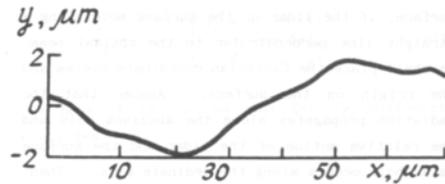
FIG. 8. The reconstructed profile of the reflecting surface
