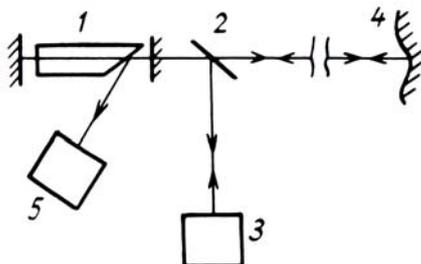
FIG. 4. Block diagram of autodyne with a frequency shift: 1) CO<sub>2</sub> laser; 2) beam-splitter; 3) frequency shifter; 4) surface; 5) photodetector.
