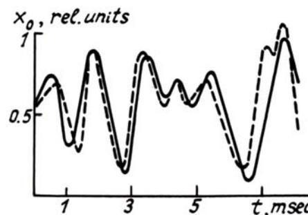
FIG. 2. Measurements of the amplitude of the oscillations. The solid line shows the measurements performed with a Doppler autodyne and the dashed line shows the measurements performed with a piezoelectric transducer.
