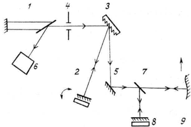
FIG. 5. Block diagram of autodyne with frequency-tunable laser: 1) gas-discharge tube of CO<sub>2</sub> laser; 2) cavity mirror mounted on a piezoelectric corrector; 3) diffraction grating; 4) diaphragm; 5) rotating mirror; 6) photodetector; 7) beam-splitter; 8) mirror on piezoelectric corrector; 9) reflecting surface.
