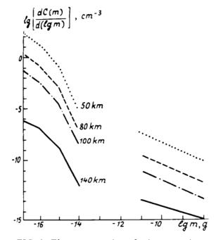
FIG. 2. The concentration of micrometeorites of different masses at altitudes of 50, 80, 100, and 140 km.
