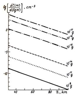
FIG. 3. The altitude dependence of the concentration of micrometeorites with masses of  $10^{-17}$ ,  $10^{-16}$ ,  $10^{-15}$ ,  $10^{-14}$ ,  $10^{-11}$ , and  $10^{-8}$  g.
