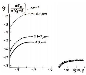
FIG. 4. The contribution of micrometeorites of different masses to the aerosol scattering coefficients for wavelength of 0.1  $\mu$ m (dots), 0.347  $\mu$ m (dashed line), and 0.5  $\mu$ T (solid line) at an altitude of z = 100 km.
