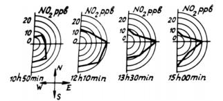
FIG. 3. The result of measurements of the nitrogen dioxide concentration as a function of the azimuthal angle in the town of Dolgoprudnyi on March 23, 1989
