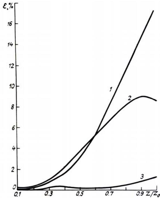
FIG. 1. Relative error  $\epsilon$ , %, as a function of relative range for vertical ground-based ranging at  $\lambda = 0.51 \mu\text{m}$ ,  $S_{\text{met}} = 23 \text{ km}$ , at  $f_{\text{laser}} = 30 \text{ kHz}$  (1), 15 kHz (2), and 5 kHz (3).
