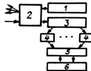
FIG. 1. Block diagram of integrated Raman-scattering lidar: 1) light source; 2) receiving and transmitting optics; 3) monochromator; 4) photomultiplier tube and discriminator; 5) multichannel integrator; 6) computer.
