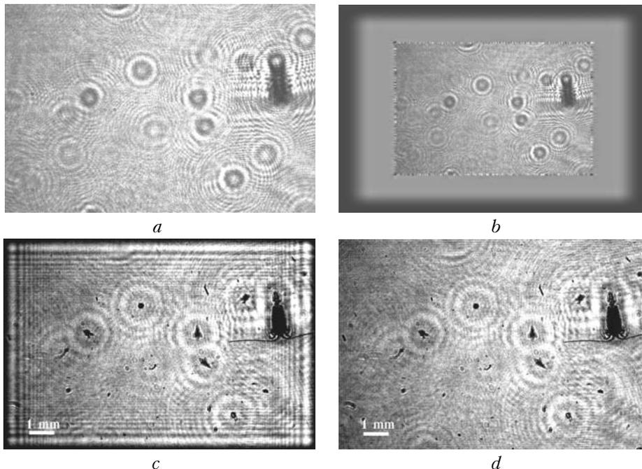
**Fig. 2.** Elimination of noises in a holographic image of a particle by preprocessing of the hologram: the initial hologram of a plankton particle (*a*); the completed hologram of the plankton particle (*b*); the holographic image of the plankton particle, reconstructed from the initial hologram *a* (*c*); the holographic image of the plankton particle, reconstructed from the completed hologram *b* (*d*).
