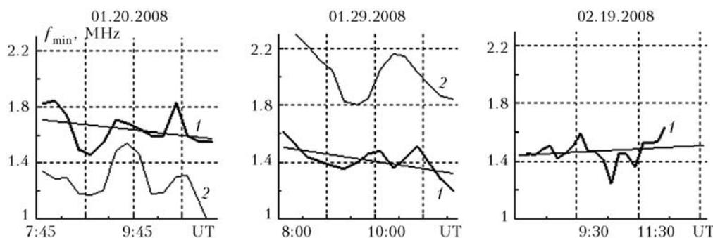
**Fig. 4.** Behavior of  $f_{\min}$  (1) and summed (over correlation region) signal (2), normalized by the squared height.
