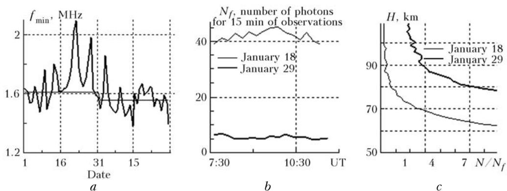
**Fig. 1.** Diurnally mean behavior of  $f_{\min}$  in winter months of 2008 (*a*), background signal (*b*), and signal-to-background ratio during lidar observations on January 18 and 29, 2008 (*c*).
