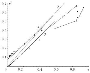
**Fig. 3.** Relative variance of intensity fluctuations of the collimated beam  $a_0 = 3$  cm (the Fresnel number  $\Omega_0 = 57$ ) in the atmosphere with precipitations: rain in the homogeneous atmosphere (simulation and calculation to MSP approximation) (1 and 3); turbulent atmosphere with precipitations, plane wave scintillation index  $\beta_{0,pw}^2 = 0.31C_{\epsilon}^2 k^{7/6} z^{11/6} = 0.1$  (simulation and MSP) (2 and 4); rain in the homogeneous atmosphere, plane wave, MSP (5).
